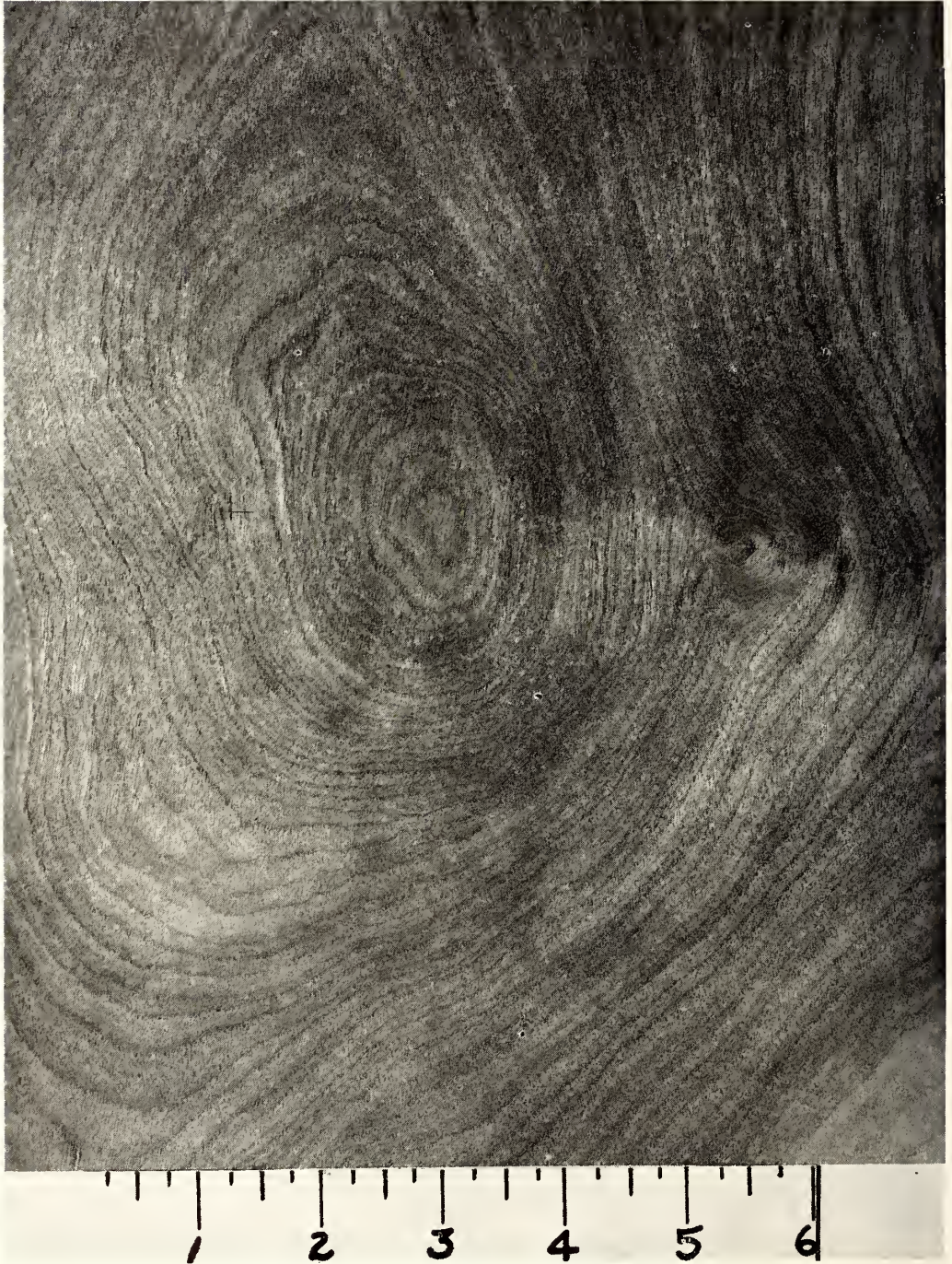
FIGURE 2-89.—Cross grain resulting from small and large bumps.
